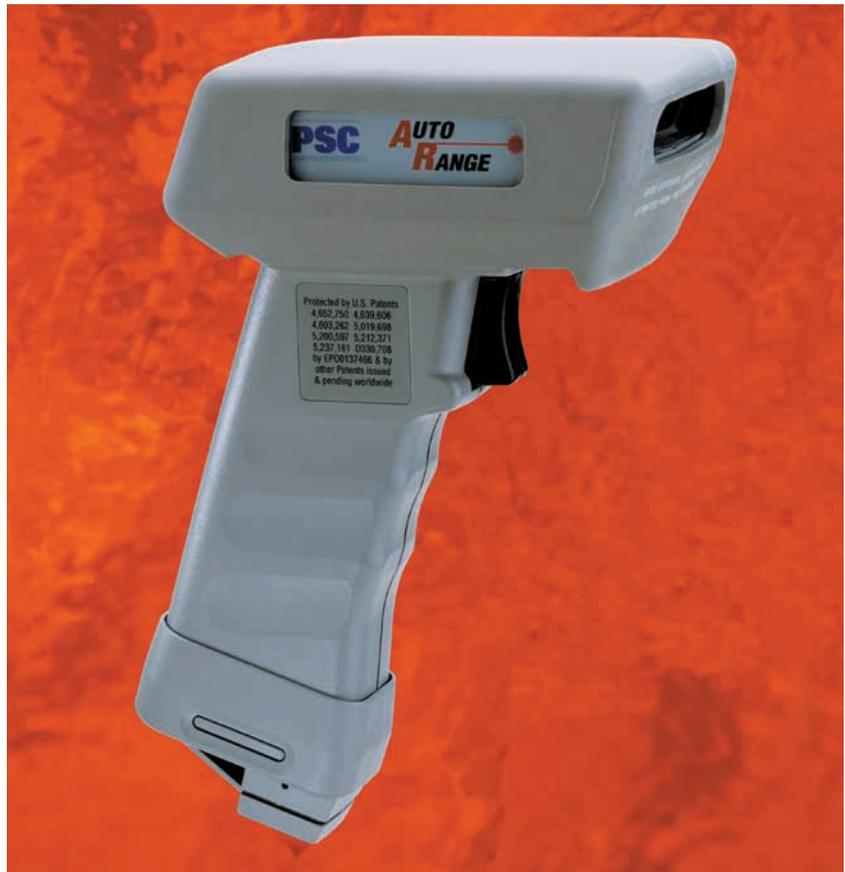
In long-range applications, the 5300IP9X scanner "reads" lower density bar codes at distances up to 40.0' (12.19m) using a long-range laser diode and long-range optical design features. A marker beam assists the operator by momentarily providing an aiming reference point on a label's surface when the scanner's trigger is initially activated.
